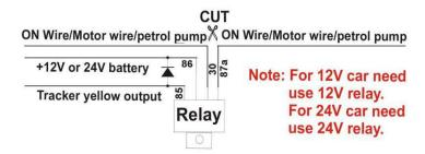
The remote turn off car engine can be disabled by "STARTENGINE\*123456", also the "CANCELALARM\*123456" command and "RESET\*123456" command can disable this command.
