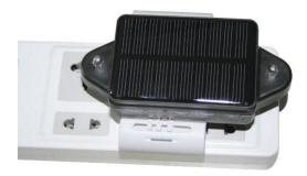
**4.2** Use Solar Charging, Place the tracker in the sunlight, the solar battery will recharge the tracker automatically, in the long distance transport or longtime tracking please install the tracker in the place with sunlight, this can extend the battery working time, but it is impossible to finished fully charging only by solar power when working.
