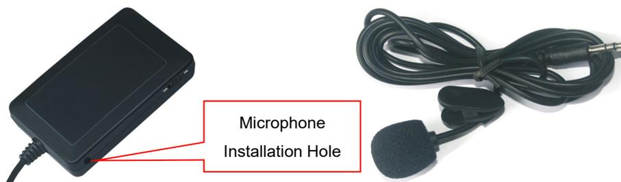
The external microphone need insert to the socket beside the wires on the case, and install the microphone in hidden place near the driver so that the tracker can have clear voice
